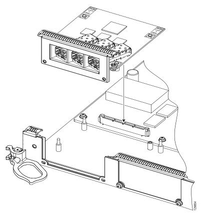
Figure 10 Side Views - Mating the Connector of the EPA to the Line Card
